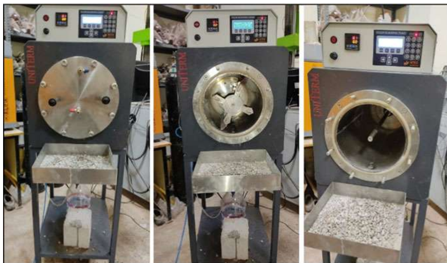
Fig. 14.2 Accelerated CO 2 capture process of RCAs
