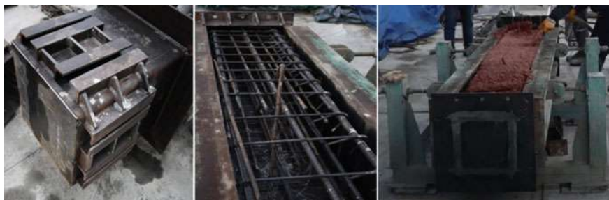
Fig. 14.6 Preparation of prefabricated geopolymer structural elements
