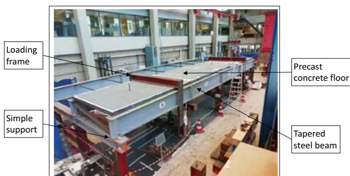
Fig. 4.4 Overview of experimental set-up [9, 13]
